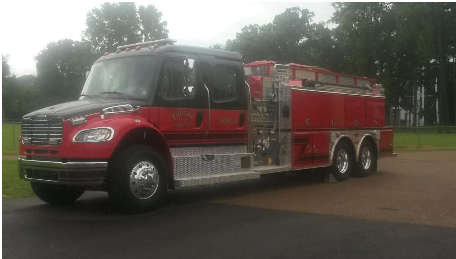
Engine 66: 1,250 GPM Hale Pump with 3,000 Gallon Water Tank
