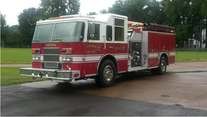
Rescue 6: 1,250 GPM Waterous Pump with 1,000 Gallon Water Tank
