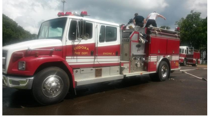
Engine 6: 1,250 GPM Hale Pump with 1,000 Gallon Water Tank
